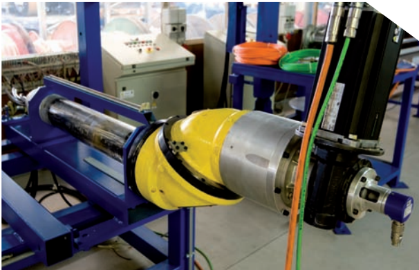
Robot wrist simulator speed 20 rad/s – acceleration 15 rad/s 2
