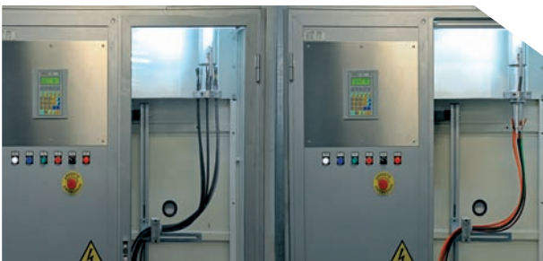
Torsion simulator – angular speed 20 rad/s angular acceleration 30 rad/s 2
