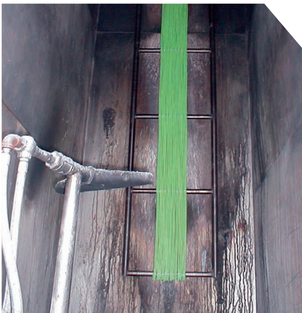
Fire-retardant tests according to CEI IEC EN 60332-3
