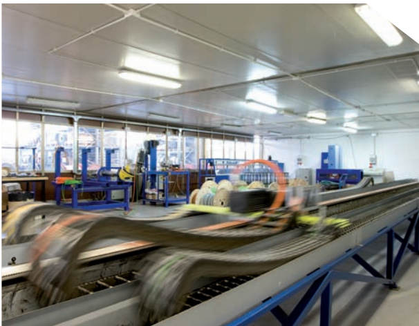
Chain with a length of 17 m – top speed 200 m/min – maximum acceleration 6 m/s 2
