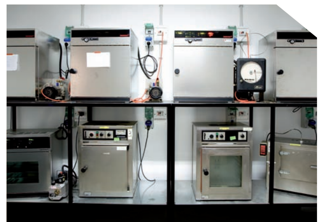
Material aging ovens
